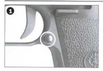
To remove the magazine, press the release located on the left side of the grip.
