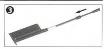
Fill the loading pipe with the appropriate 6 mm plastic BBs. W orks best with Cybergun's BBs 0.20 g (item# 71100). Fit the end of the loading pipe to the top of the magazine. It should adjust tightly. Using the rod provided, gently push all the BBs into the magazine.
