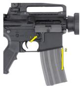
1. Press the magazine catch button to release the magazine.
