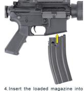
4. Insert the loaded magazine into the rifle.
