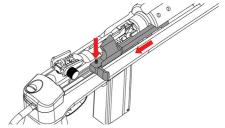
When the rifle is empty, user can pull the charging slide backwards and press the slide stop indicated by arrow to lock the charging slide and change the magazine.
