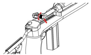
For the adjustment of rear sight, rotate the thumb screw indicated by arrow forwards or backwards to desired position.
