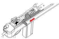
Pull the charging slide backwards to load the rifle. The BBs in the magazine will be loaded into the chamber automatically once the charging slide been released.
