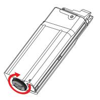
3. Replace the end cap and tighten it in clockwise direction snugly. \*For safety reason, release all the pressure inside the magazine during storage.\*
