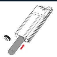
2. Insert the CO2 cartridge into the magazine.
