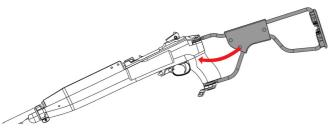
The steel made wire stock can be folded in the direction as the arrow show.
