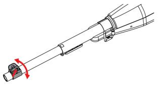
For the adjustment of front sight, loosen the hex screw indicated by arrow first, then rotate the front sight to desired position.
