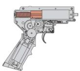
In this situation, the piston is stopped in the middle of the shooting cycle. The spring is now being compressed and it will cause damage to the spring in long run.
