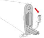
2. Pull out the wiring from the buttstock.
