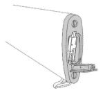
4. Insert the wiring into the buttstock. Make sure all the wiring stayed inside the buttstock then close the cover.
