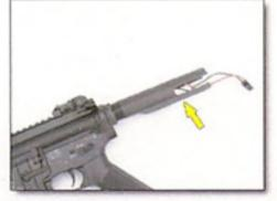
Remove the stock from AEG, then pull out the wires in the pipe.
