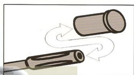
Always attach the protective plug to the gun muzzle.
