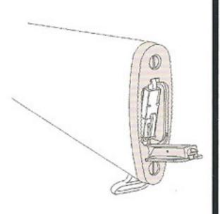
4. Insert connectors and cords in the stock. Close the cover when the battery and cords are set in positions.
