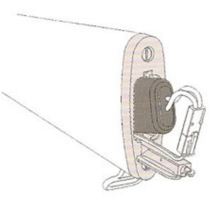
3. Insert the battery in the stock and connect connectors.
