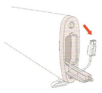
2. Pull out the connector from the butt stock.
