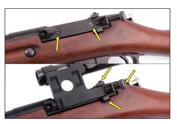
Place the mount base on the rifle as shown and tighten it with 2 screws. And then put the scope on the mount base and lock it in place with 3 screws as shown.
