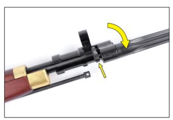
Turn the bayonet 90 degrees and the locking button will be released to lock the bayonet in position.
