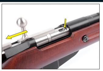
Pull the cocking handle backwards until gas charging valve on cylinder is shown. Then fill the cylinder with 134A and make sure there is no leaking.
