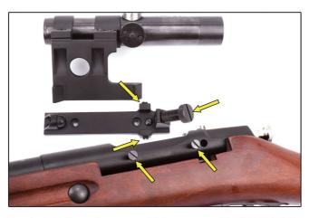
For installation of scope which comes with KA-AG-171. First, release the 3 screws on the mount base and take the scope off as shown. Ant then release the 2 screws on the rifle as shown.
