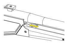
o Excessive hop up (Push the lever forward.)
