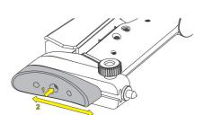
Loosen the hex screw indicated and then you can adjust the butt pad vertically. Fix the hex screw back on once finished.
