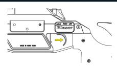
3. Make sure the safety selector is on "FIRE" mode, then pull trigger to shoot.
