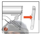
Press the tabs down to release the buttpad from the stock.
