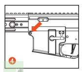
Unscrew front pin with hex key. Tap the front body pin out until the upper receiver disconnects.
