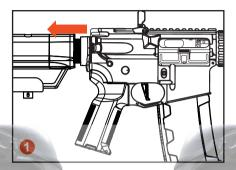
Pull the charging handle back to move the bolt plate back, thus exposing the hop-up adjustment dial. Hold in place while adjusting the hop-up.
