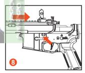
While sliding upper receiver back into place, pull changing handle as in Step 6. And hold down the lower end of the mock bolt release so it does not block the path of upper receiver.
