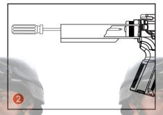
Look into the buffer tube with a light source to spot the Phillips screw. Use an long Phillips screwdriver, resulting in removing the buffer tube, screw and washer from the receiver. Be careful not to pull or cut the wire.
