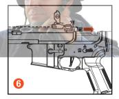
While sliding upper receiver forward, draw back charging handle to work it past obstructions on top of the internal gearbox.
