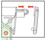
Connect the battery to the connector. Slide the battery into stock compartment. Close buttpad.
