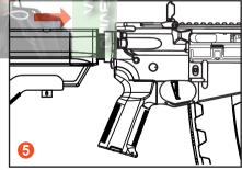
When hop-up is fully adjusted, release charging handle to move the bolt plate back to its original position.
