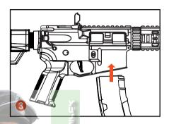
Press the mag release button to remove magazine.
