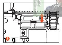
Turning the dial downward will cause the BB to float upwards, whereas turning the dial upward causes the BB to fall downward
