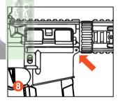
Align the front pin with the lower receiver. Push in the pin to secure both receivers.
