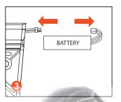
Remove the battery. (See battery installation page)
