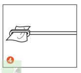
Take a 1" cleaning cloth and attach it through the loop-end of the cleaning rod.
