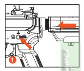
Make sure the selector switch is set to safe & fully retract the stock.
