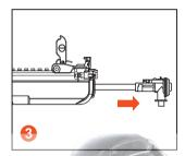
Slide the inner barrel and hop-up assembly out of the upper receiver.
