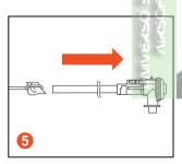
Push the cleaning rod through the inner barrel from front to back.
