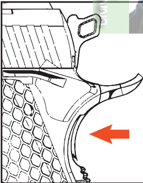
Grip safety is a lever situated on the pistol grip which must be actuated by the operator's hand. Only by naturally grasping down can the pistol fire.
