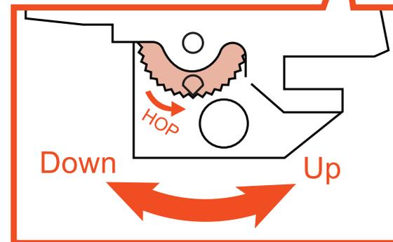
The hop-up system can adjust the trajectory of BBs fly up or downward.
