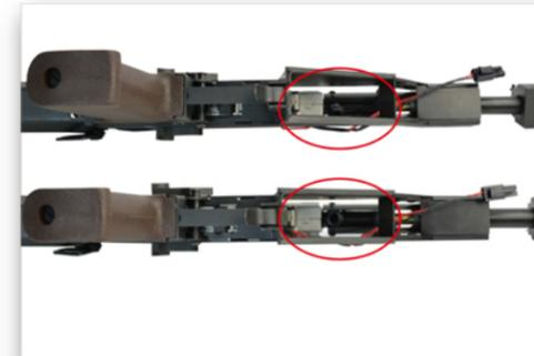
2. First, secure the gearbox screws, then install the gearbox wires onto the motor. The red wire should attach to the red connector and black wire to the silver connector, then tighten the motor screws.
