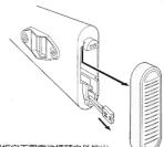
將托底板向下壓電池插頭向外拉出 Push down and take off the butt-plate, then take the wire,battery connector and fuse container out of the buttstock.
