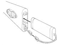
將電池插頭接合後再放入電池 Connect the battery to the battery \ connector carefully.
