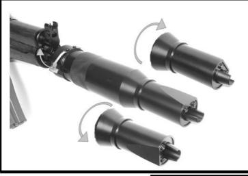
To adjust the position of silencer muzzle, pull up the spring plate and rotate PBS-4 right or left.
