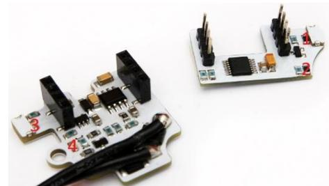
Optical sensors and IR LED diodes work in pair as a barrier switch. If the trigger is at rest, it obstructs vision between the trigger sensor and diode. Once the trigger is pulled, the infrared radiation flows from the diode to the sensor signaling that a shot should be fired. This way the mechanical trigger lock can be retained. It also allows for the “hair trigger” modification (see more on page 7).
