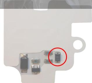
When selector is in “SEMI” position, selector plate should not be over the optical sensor. Sensor then will have black body of the lower receiver in front of itself, reflecting little infrared and thus indicating “SEMI” selector position. In some replicas even in “SEMI” position selector plate will cover part of or whole sensor. In that case selector stickers with thin or thick black belt should be used.
