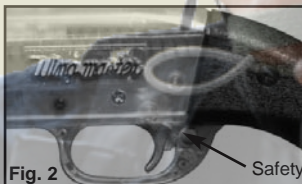
Fig. 2 PUSH IN FROM LEFT FOR "ON SAFE" PUSH IN FROM RIGHT FOR "OFF SAFE"
