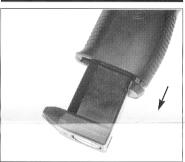
When shooting is over, check magazine is empty and safety back in the locked position, as indicated on the picture.
