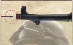
2. Turn off the hop up by moving the hop up lever all the way towards the normal setting. Use the slanted end of the cleaning rod
