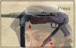
2. Press the stock release button 3. Rotate the stock until the to fold the stock
