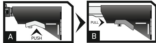
Some models have an adjustable stock adjustable stock that can be set in 4 or 5 positions. To modify the stock's position, press the lever and push or pull the stock.
