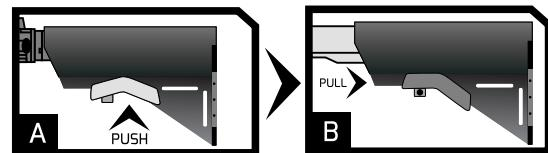
Some models have an adjustable stock adjustable stock that can be set in 4 or 5 positions. To modify the stock's position, press the lever and push or pull the stock.
