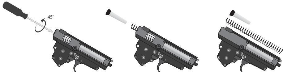
1 Use a screwdriver to gently push the spring guide inside the gearbox. Rotate the guide by approximately 45 degrees, until you feel the spring's resistance.
