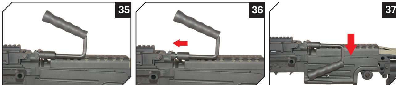
Depending on the version of the replica, it has a convenient carrying handle. Due to the weight and dimensions of the replica, the handle allows you to carry it more comfortably. The handle can be folded or unfolded. Just pull it back and rotate it up or down [36, 37].
