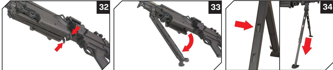
The replica has an integrated, adjustable bipod. To unfold the bipod, pull the legs towards you [32] and fold them down [33], allowing the spring to spread them out to the sides. Both legs are height-adjustable. To do that, use the button in the guide [34]. It can be set in 3 positions. To assemble the bipod, repeat the steps in reverse order.
