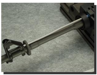
Align front sight post with outer barrel, and insert two Front Sight Post Knock-Pins (BR-010) to secure the front sight post.
