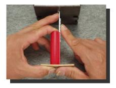
Assemble Piston Head by first gluing Piston Head Bumper (black, flat rubber ring, CU-008) to Piston Head (CU-007) using instant glue. Then install Main O-Ring for Piston Head (CU-010) around the outside of piston head, and Small O-Ring for Piston Head (CU-009) inside the opening in front of the piston head. Refer to photo. Apply sufficient amount of Systema cylinder grease to where small o-ring is fitted.
