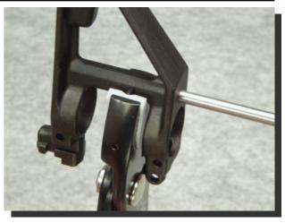
Insert front sight post over barrel. The gas pipe should pass through the corresponding hole in the hand guard cap, barrel nut assembly (hole prepared in last step), and finally into the upper receiver.
