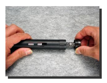
4. Installation of Inner-Barrel Assembly Insert Inner-Barrel Assembly (ASS-BR-04/05) to upper receiver, noting the orientation of the BB feeding opening, as shown.
