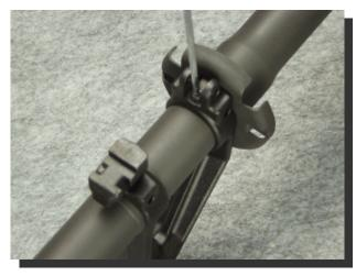
Fix Front-Sight Post Swivel-Ring (BR-032) and press-fit (or using pin punch) Front-Sight Post Swivel-Ring Pin (BR-011).
