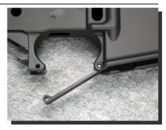
Next, press-fit Trigger Guard Set Pin (LR-018) with Teflon-based pliers as shown.
