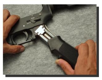
Once the grip is fully inserted, through the opening at the bottom make sure the positive motor wire is routed towards the side of the motor's bottom mount point. There is a small notch on either side of the grip end for the wire to rest. If the wire do not rest in said groove, it will be damaged.
