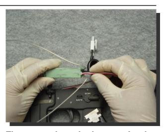
Then remove the stock tube cap, and push the battery plug, coiled cord, and the switch device (in this order) into the stock tube. Replace stock tube cap when done.
