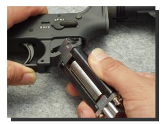
Once the motor is in-place, insert the Motor Fixing Pins (LR-023, x2). If the pin do not fit in smoothly and tapping / hammering is required, make sure the motor is properly and evenly supported first. A piece of board under the motor to distribute the pressre would work. This is important because the motor is a structural part of the PTW, and it (or its joint to the lower receiver) must not be deformed.
