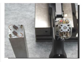
9. Install Grip and Grip End Gently slide the Grip (LR-022) over the motor, ensuring the motor wires do not get squeezed or pinched between the grip and the motor.
