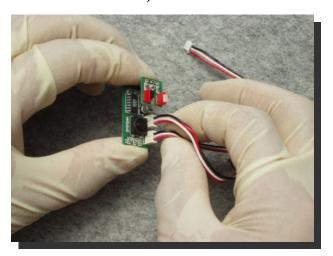
Finally, insert the Electrical Control Unit very carefully into the gearbox. Pay extra attention to now each control cable exits the gearbox from the side. You should try to arrange the cables as shown.
