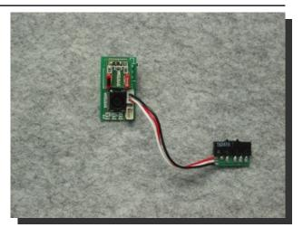
Connect one end of the Control Cable (EL-004) on to the lower socket of the electrical control unit. Note the use of rubber glove.
