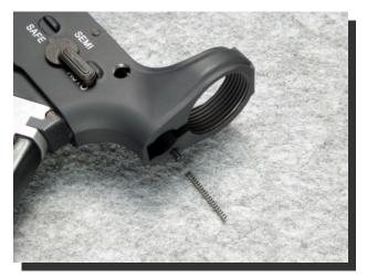
Finally, screw stock tube into lower receiver. Pay attention to the positioning; the front end of the stock tube should not protude from the lower receiver. If the stock tube is too far forward, the receivers won't close. Typically the front of the stock tube should still be about 2mm recessed.
