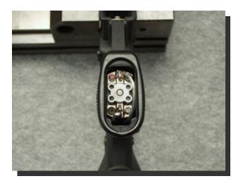
Next, place Grip End (LR-025) over the bottom opening of the grip with the correct orientation (see picture) and fasten the grip end to the motor by using the 4 Group End
