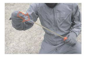
While keeping a firm grip on the magazine and loading tool, insert the provided acrylic rod into the feeding tube with your other hand. Use the acrylic rod to push the BBs through the loading tube into the magazine. You should not need to apply excessive force. Repeat the loading process if you need to load more BBs then the loading tube will hold. When a resistant builds up while pushing the loading rod down, your magazine is full.
