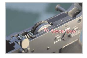
gears, tap the trigger lightly until all of the sector gear's teeth rotates inside the lower receiver (as shown), before you attempt to close the upper receiver.
