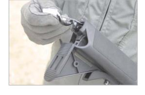
Insert battery as shown, ensuring the connectors on both the battery-side and the stock-side lines up, then carefully connect them. The connectors are polarized so they will only fit together in one direction.
