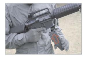
Depress the bolt-catch release pad to simulate releasing the bolt of a real M16. Although you will not feel a bolt slamming forward in the Professional Training Weapon, this action is still required as an electrical sensor located behind the bolt-catch will prevent the
