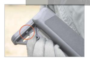
Then Locate the two notches that secure the battery compartment cover (butt plate) to the stock. Lightly squeeze them together to remove the battery compartment cover.
