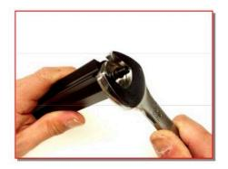
■Installation of the Cylinder Head Assembly
