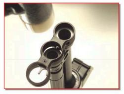
■Installation of the fixed front sight post sleeve.
