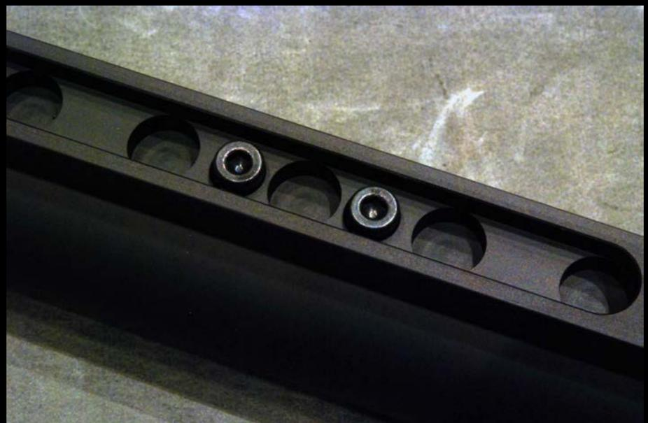
However, in the event that the screws are over tightened, the Recoil Pulley Gear Stand may warp its shape. The goal is to aim for around the 9 O'clock position.
