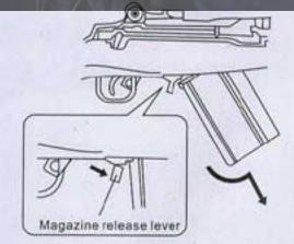
· Removing the Magazine Press the magazine release lever to remove the magazine.
