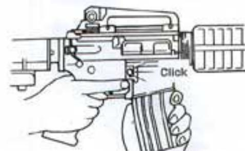
**CAUTION** Confirm that the safety lever is set to the Safety position and don't place your finger on the trigger.
