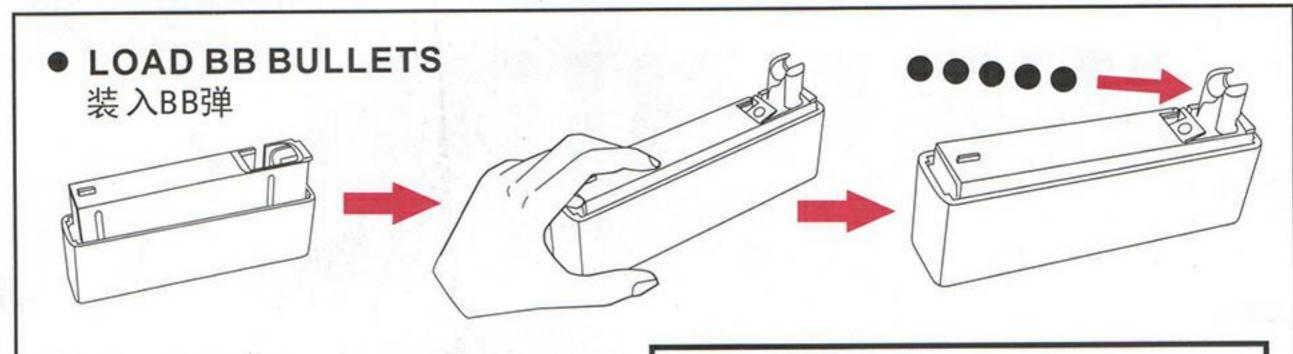
PRESS THE MAGAZINE AND LOAD THE BB BULLETS
