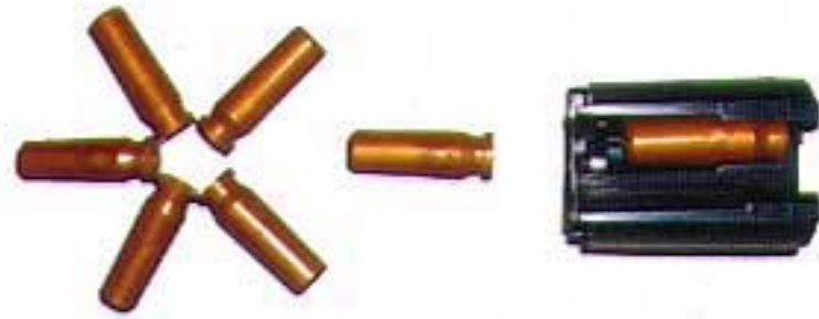
B2. Load maximum five shells into a magazine.
