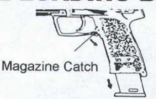
Press the magazine catch to release the magazine.
