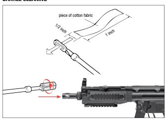
Put the safety ON SAFE and remove the magazine and the battery. Prepare a thin rod with a length of approx. 16 inches. Attach a piece of cotton fabric to its end and clean the barrel with some
