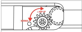
Open bolt to adjust the Hop-Up system.
