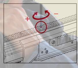
■ Gradually rotate the allen wrench (included in box) forward and fire a round or two to see the effect.
