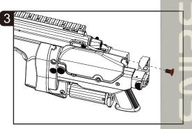
Use the allen wrench (included in box) to tighten the screw.
