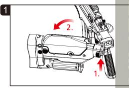
Push the stock upward to unfold.
