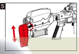
Push the button to adjust the buttstock pad vertically.
