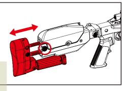
Press the button to adjust the buttstock pad horizontally.
