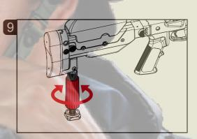
Adjust the height of the monopod by rotating the handle.
