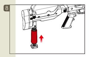
Press the monopod upwards to lock it in place.
