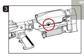
Release the screw to adjust the cheek piece.
