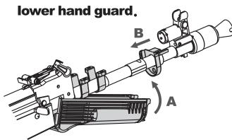
Install the AK Scout Mount instead the upper hand guard and cleaning rod.
