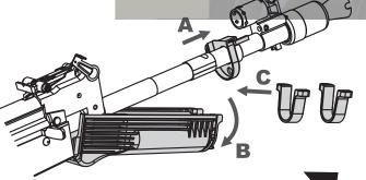
Put the U Clamps under the barrel and then install the
