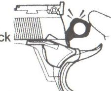
□ Half Lock is referred to that the hammer stays between the Full Lock and Hammer Down. Under this state, it is of safety.
