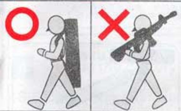
When you carry the air gun, attach the protective plug, set the selector lever to the Safety position and put it in a case or bag.
