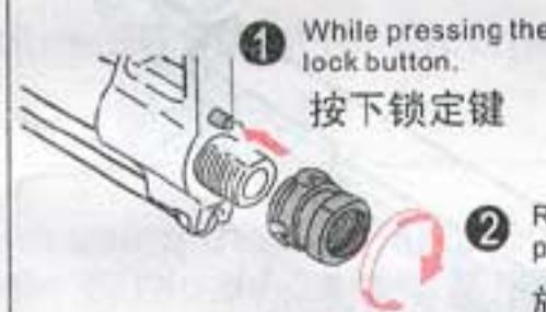
The Multi protector is fixed by reverse thread as in the case of the real gun.
