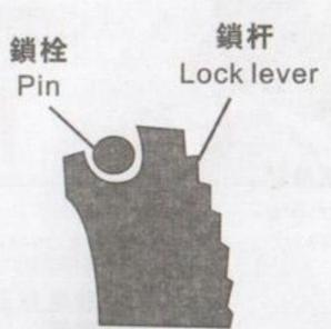
NOTE: At the locked state, the lock lever tip catches the pin.
