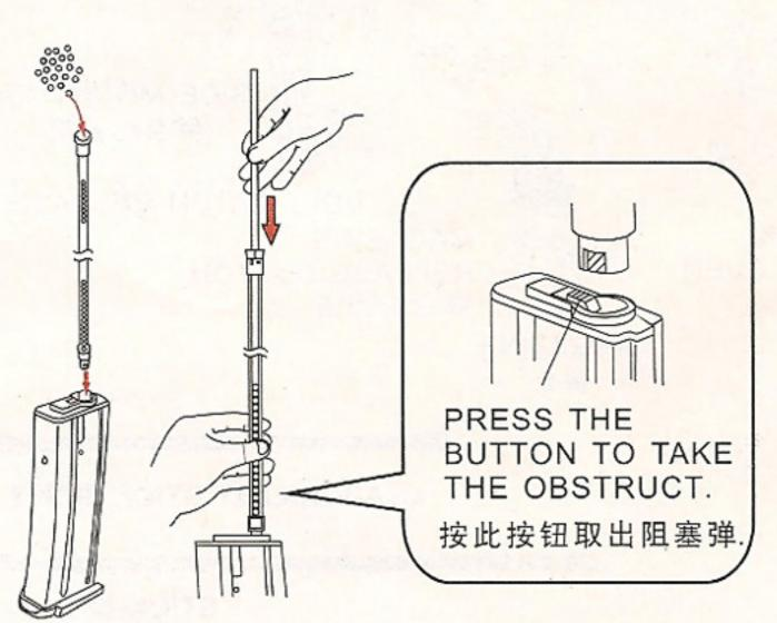
INSERT THE STICK INTO THE TUBE TO PUSH THE BULLETS INTO THE MAGAZINE.
