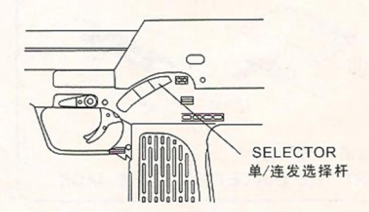
NEVER OPERATE THE SELECTOR WHILE PULLING THE TRIGGER. OTHERWISE, MALFUNCTIONS MAY OCCUR. PULLING THE TRIGGER WITH THE SELECTOR BEING SET TO SAFE MAY DAMAGE THE GUN.
