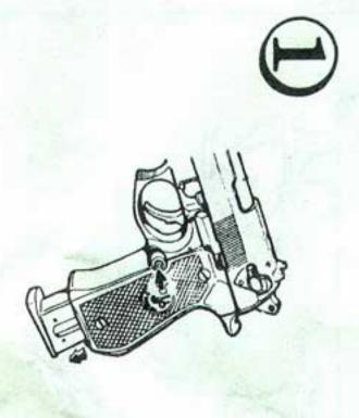
Press the catch to un-load the magazine as shown.
