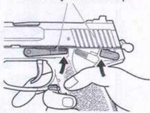
When hammer is not pulled back, single safey is available at the front lever
