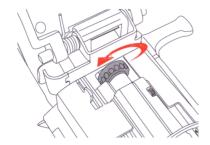
With hop up, BB pellets are able to extend its trajectory with revolution Adjust with 2mm wrench.
