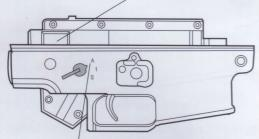
Make sure the fan-shaped gear in the body is totally matched with the selector gear on the gear box now.
