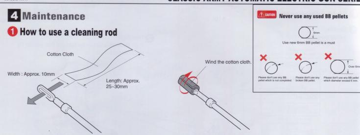
Cut a cotton cloth to the size as shown above and insert one end into the hole in the rod. (Adjust the length of cloth for smooth entry into the barrel.)
