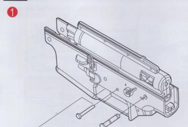
Pry up the body at the upper-left side of the selector with a ø6 screw driver. Then, turn the selector clockwise until it point to the bottom.
