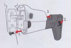
4 Insert the battery into the stock.
