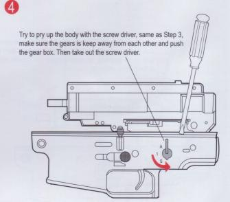
Pry up the body again and adjust the position of the selector by turning it anti-clockwise until it pointed to letter 'A'. Check the both side of the selector is correctly functioned or not.
