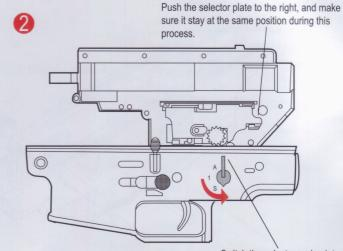
Switch the selector and point to the bottom.
