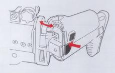
3 Take out the connector and connect it with the battery.
