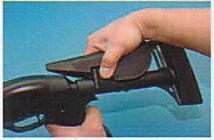
Push the button on the stock, slightly turn it to the right. Push the stock forward until it is locked in the concave.
