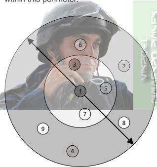
In noisy environments, simply walk close to the person you wish to talk to. The NIB technology will softly fade in and out (5-10 m radius) and allow communication with people who are close. Stay within 3-5 m radius for optimal communication signal.
