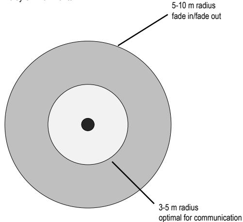
The NIB technology enables wireless communication within a 10 m radius. Full duplex communication for up to four people within this perimeter.
