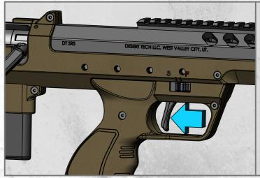
Pull the trigger to realease the spring guide in the buttplate. Make sure the spring guide is sitting in the correct position.
