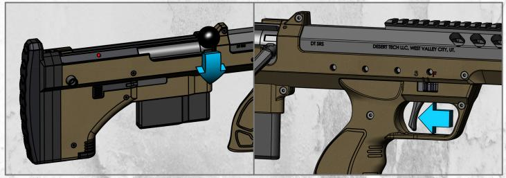
Lock down the bolt handle to lock the bolt. You can check the primming indicator: it should be now in red color, indicating the gun is ready to fire. This feature isn't available for lefty SRS.
