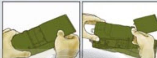
1 With back of radio case facing you, push the cover toward the angled top of the radio case.
