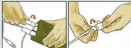
1 Assemble the antenna on the case by loosen it at anticlockwise, install the antenna connectors by twist it clockwise.
