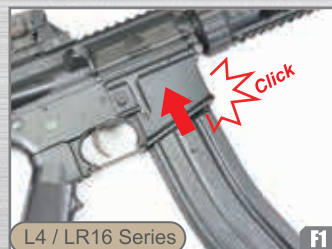
Tilt and insert the hook into the magazine socket. (show as red arrows)
