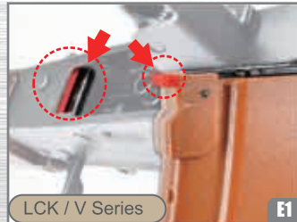
Tilt and insert the hook into the magazine socket. (show as red arrows)
