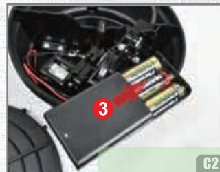
Install 3 AA alkaline batteries into the battery box. Trun the power switch ON. Put the butt plate back and fix the screw.
