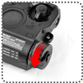
1. Unscrew the battery cap.
