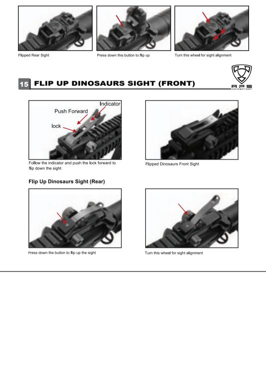
Two way rear sight (small hole for aiming long range and big hole for aiming close range
